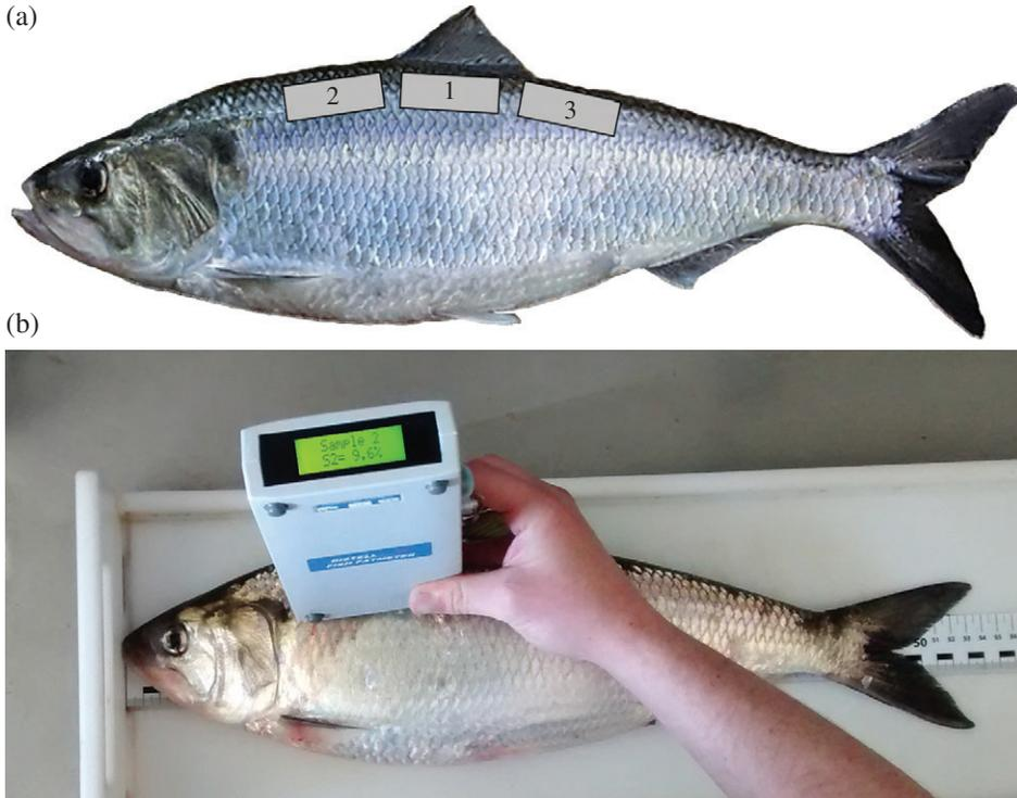
FIG. 1. (a) Side-view of an *Alosa sapidissima* indicating positions (1, 2 and 3) where fat-meter readings were taken and (b) fat meter in use at position 2.
